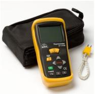
These single input K-Type thermometers offer high accuracy and fast response times. Ideal for industrial and laboratory use.
